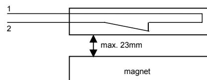
**Built-in mounting:** For the built-in contact version, holes (8 mm and 0.2 mm) have to be drilled for the switch and magnets. The switch must fit easily into the hole but tightly enough so that it cannot be removed without using technical means. To avoid damage, do not use force when installing the contact. Contacts must not be built into either ferromagnetic materials or materials with a ferromagnetic core.
