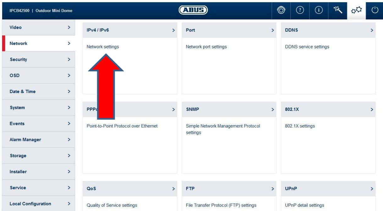
In the menu item IPv4/IPv6, set a fixed IP address that is compliant with the existing network address range or check the box for DHCP. The address is then assigned by your router:
