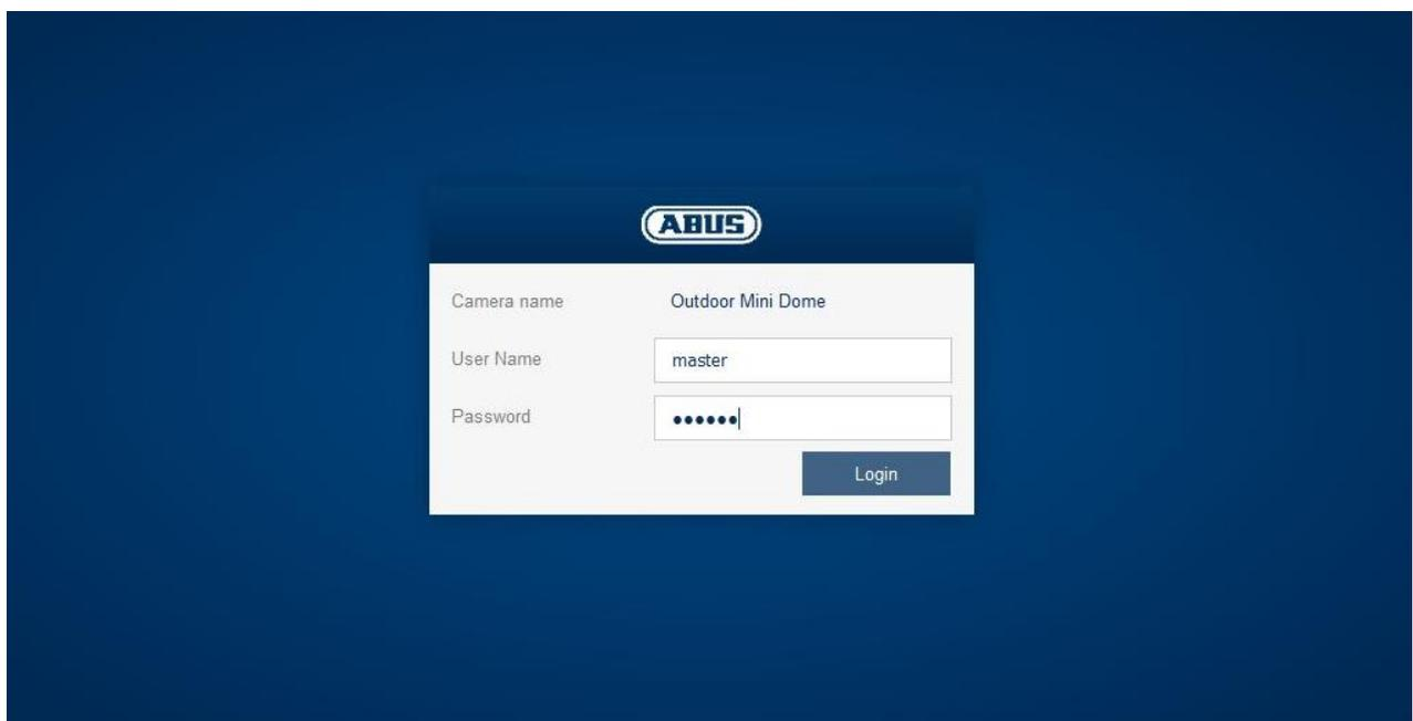
Unlike in the configuration process, you must log in as a user (this time with the user name **master** and password **master**). In the screen below, it is possible to create other users that can be logged in for searches. Click on the settings menu in the top right corner:
