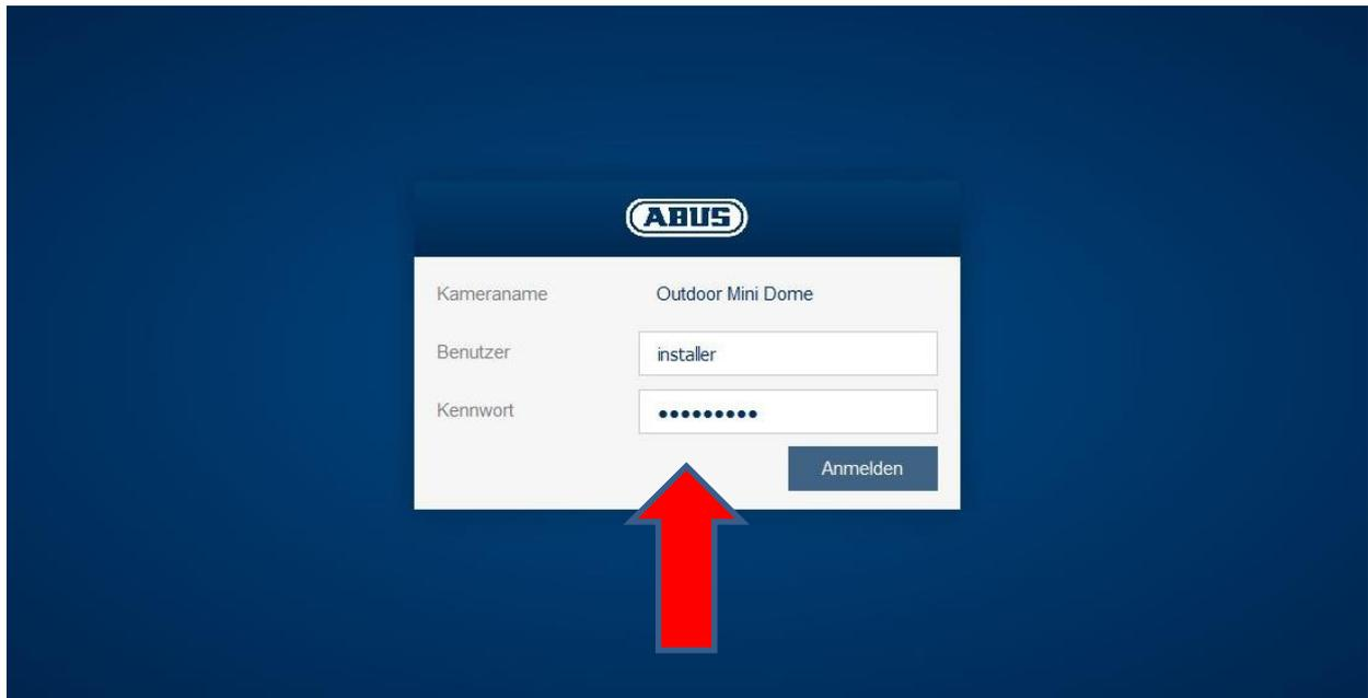
The first time the camera's live view is opened, the user name and password are both *installer*. Click on Settings:
