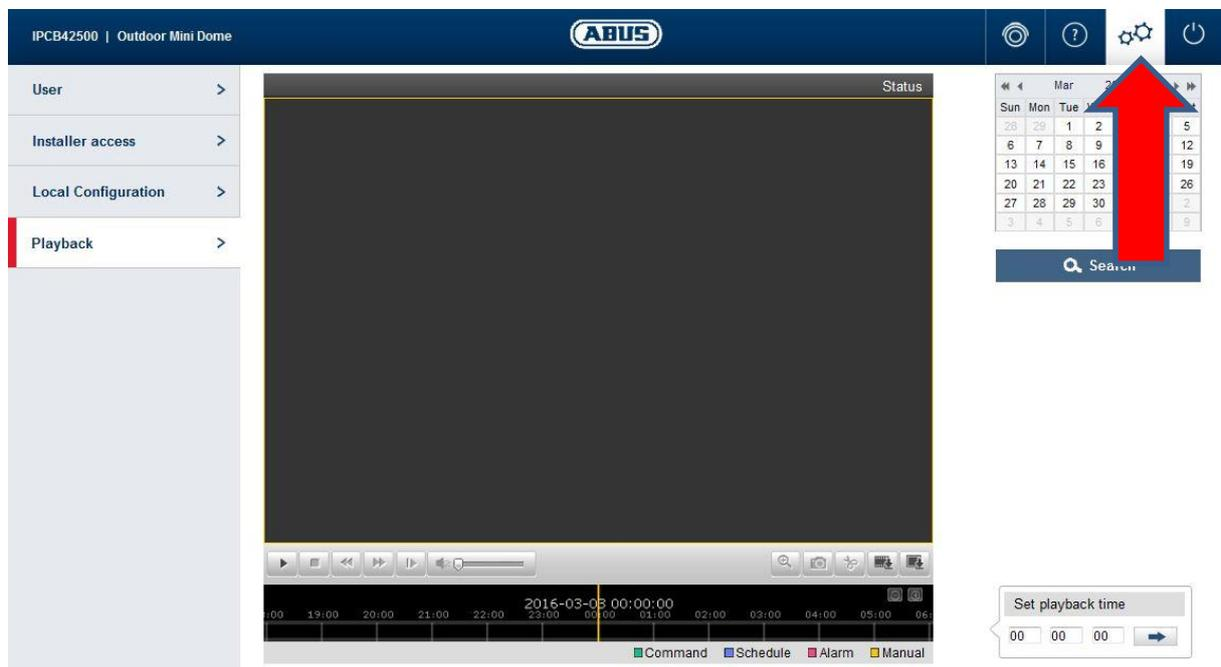
All videos and images can be displayed in the **Playback** tab depending on whether images or videos have been set in the alarm system (see page 10). Please note that the length of recordings depends on the SD card size, quality setting, type (video or image) and the frequency of trigger events. This menu also gives you the option of saving videos and images from the SD card on your computer:
