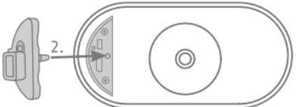
Insert the new red cover that came with the solar panel so that the new cover sits completely plane to the back of the WLAN Battery Cam and ensures waterproofing.
