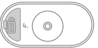
**Important:** To ensure the required watertightness, the new cover must sit flat and centered all around with no bulging.
