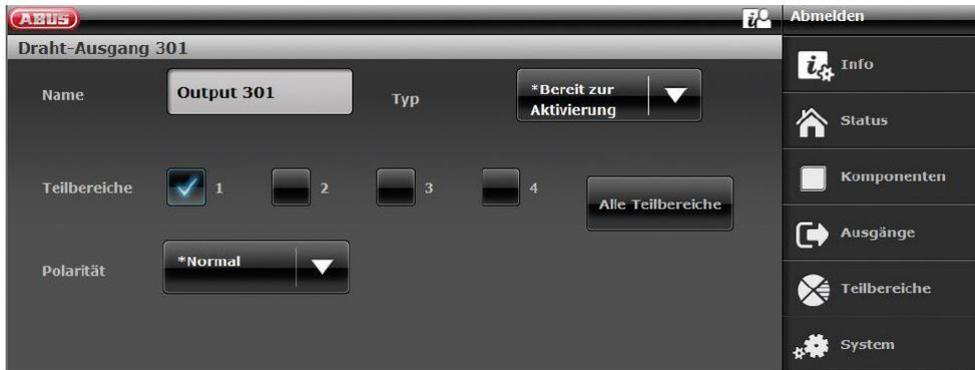
Configuration of the wired output 302 (relay 02) for the activation on the Secvest
