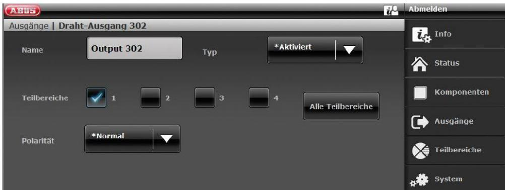
Configuration of the output mode for each partition on the Secvest (not pre-configured)
