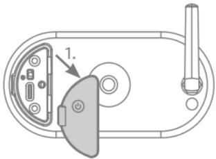
On the back of your Battery Cam Pro, completely remove the original red cover by completely pulling out the rubber anchor element of the red cover.
