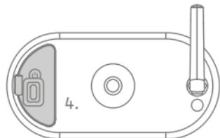
**Important:** In order to guarantee the required water-tightness, the new cover must be flat all around and be positioned centrally without bulging.
