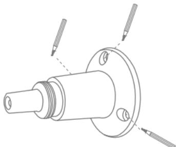
Mark the position of the required 3 drill holes at the desired location using the drilling template or wall bracket and a pencil or similar instrument. You can unscrew the bracket parts to do this. When choosing the location, also consider the maximum cable length of the solar panel.
