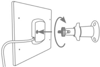
Turn the ball joint of the bracket with the thread into the corresponding opening on the back of the solar panel. Tighten the enclosed union nut so that the ball joint and solar panel are securely connected.
