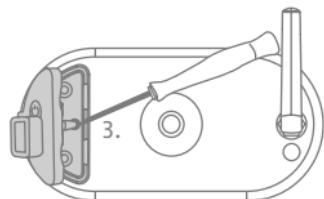
**Tip:** You can use a narrow object, for example, a very small screwdriver, to position the small rubber anchor element on the inside of the new cover. Make sure that the anchor element holds the new red cover securely.
