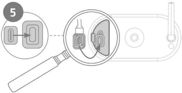
Connect the USB-C connector of the solar panel cable to the USB-C port of the Battery Cam Pro. Make sure that the plug is seated correctly and firmly. Also make sure that the rubber seals are seated correctly to ensure water-tightness.
