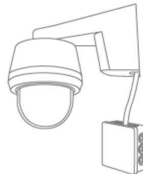
1. Separate the wall plate of the bracket from the camera using the Allen key provided. Mark the position of the required 4 drill holes at the desired location using the drill template or the wall plate and a pencil, for example. Drill the holes and insert the dowels provided. Secure the bracket with the screws provided.
