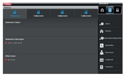
If there is an error in the system, the information on this is displayed as follows (in this example a magnetic contact is open):
