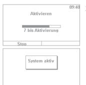
2. If the bey is then pressed, the system is completely armed. As mentioned previously, the system is armed only once the delay time has expired as programmed by your installation contractor.
