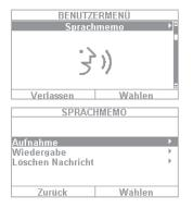
This function is used to leave someone else a message ("Memo function"). Record a short reminder, for example, and then arm the system. The next person to disarm the system is notified with the text "You have a message" and a corresponding symbol. Select "Recording" to record a 30-second message and then save it. Any user can delete this message after it has been played back. This function can be completely disabled in consultation with the specialist installation contractor.
