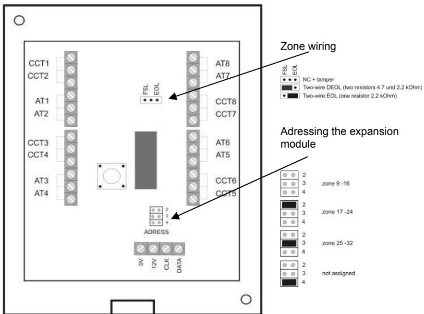
The 4 wires from the communication bus of the alarm panel are connected at the data BUS as described in the installation instructions of the alarm panel. Additional modules are connected in parallel at this BUS. The zone ranges are differentiated by the addressing of the modules. You must also set the type of zone wiring. The zone types from the alarm centre and the expansion modules may be different.
