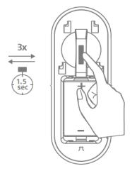
Press the Tamper-button 3 times within 1.5 seconds and the Status-LED on the base unit front will flash 3 times
