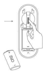
Press and hold the tamper button while inserting the battery.
