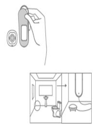
Mount the base unit to the wall by using the adhesive strip
