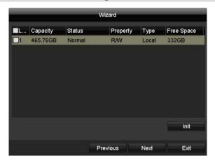
To set up a hard disk drive, enable the 'checkbox' with a left click and then click on **Init.**
