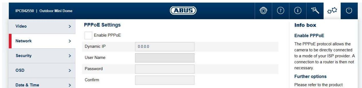
The PPPoE protocol makes it possible to connect the camera to a provider modem directly. An additional router is not required.
