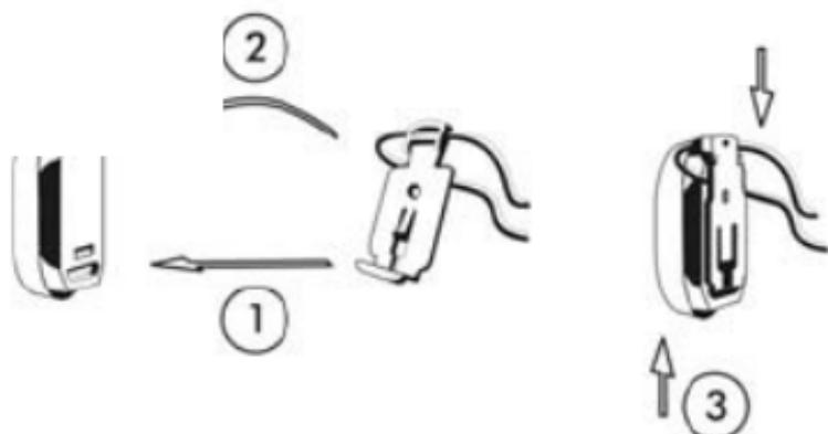
Insert the lower end of the lanyard clip into the lower housing slot (1).
