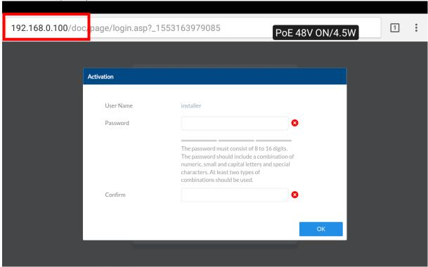
After activation, you can proceed directly with configuration and setup of the camera in the web browser. Alternatively, you can also use the pre-installed IPCam Plus or the manufacturer-independent IPC Test App.
