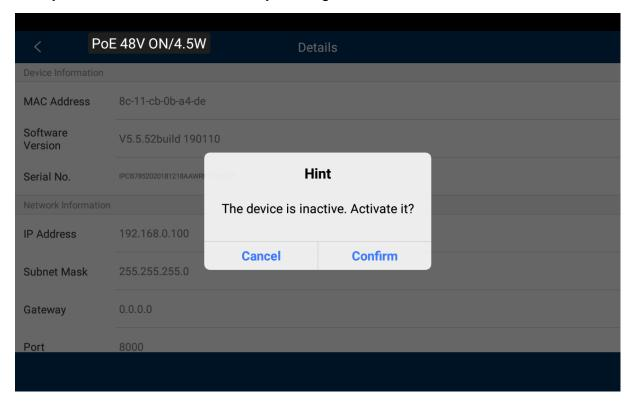
After activation, you can proceed directly with configuration and setup of the camera in the iDVR Plus App. Alternatively, you can also use the pre-installed IPCam Plus or the manufacturer-independent IPC Test App.
