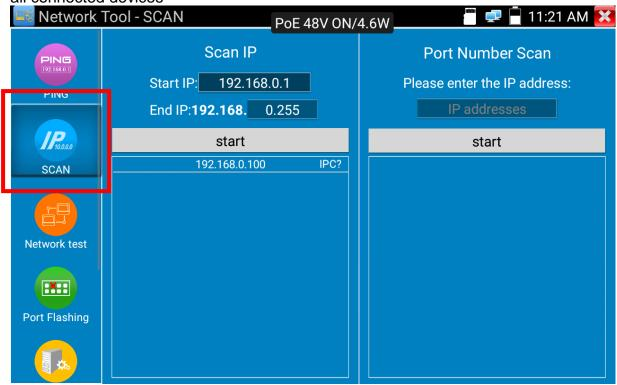
If this search does not succeed, as the address range is unknown, you can activate the DHCP function of the test monitor to assign an IP address from the user-defined range to the connected device.
