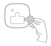
Remove the safety strip from the battery compartment.
