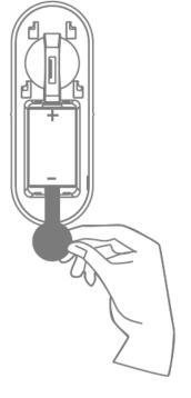
Slide the base unit from the mounting plate and remove the safety strip from the battery compartment
