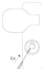
When the cylinder body has been installed in the lock, secure the basket (3.2) to the shaft with the motor (3.3) using 6 screws.
