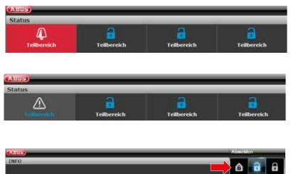
Acknowledge an alarm by selecting the red partition and confirming the prompt for whether the alarm should be acknowledged.
