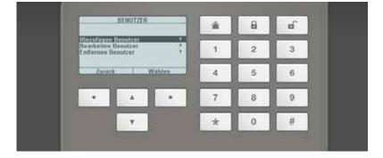
Under "**Keypad**" you will find the "Virtual control panel" function. You can use this function to view the Secvest menu via the web interface and assign a created user to a remote control, for example. Move the virtual cursor keys using the mouse and go to the "User" menu. Further options are displayed there.
