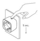
Keep pressing the Button on the socket for more than 5 seconds (the flash interval of the Status LED is now accelerated)
