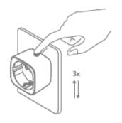
Press the Button on the socket 3 times
