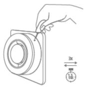
Press the Network-button 3 times within 1.5 seconds and the Status-LED will flash 3 times
