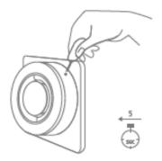
Press and hold the network button for 5 seconds.
