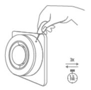
Press the Network-button 3 times within 1.5 seconds and the Status-LED will flash 3 times
