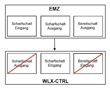
Only the Arm Input is connected to the Arm Output of the alarm panel. This involves using the alarm panel to lock the wAppLoxx Pro Control in its "armed" position until the alarm panel unlocks it again. It is not possible to use the wAppLoxx Pro Control to "disarm" the system here. You can only actuate the connected wAppLoxx Pro Cylinders when the alarm system is unarmed.
