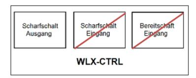
Only the Arm Output of the wAppLoxx Pro Control is configured, although it is not connected. This makes it possible to lock the cylinders with an Arm command until a valid Arm/Disarm medium is presented.
