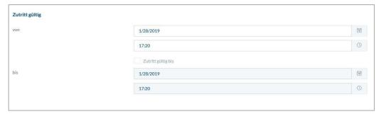
This section allows you to define an individual validity period for users. The defined validity period applies to all permissions in the system, for access to both the relevant wAppLoxx Pro Cylinder and the web.
