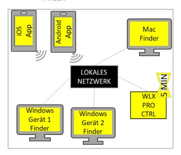
The wAppLoxx Pro Control will be ready to exchange security keys with a device on the local network within the first five minutes. By restarting the wAppLoxx Pro Control (e.g. by pressing Reset A), this time can be restarted.
