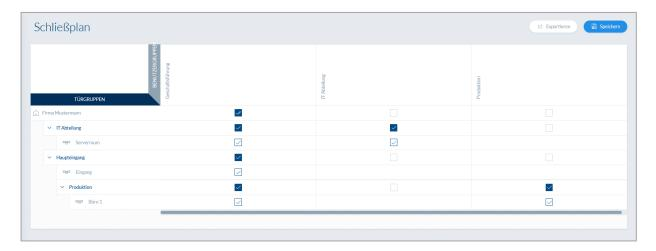
Authorisations are assigned in the wAppLoxx Pro System using a locking plan matrix. The assignments and access rights are issued simply by clicking on the relevant checkbox. The following selection options appear when you click on one of the checkboxes:
