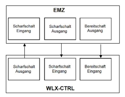
The Arm Input, Arm Output and Ready for Arm options are connected to the alarm panel. This makes it possible to "arm" and "disarm" the system using the wAppLoxx Pro Control.
