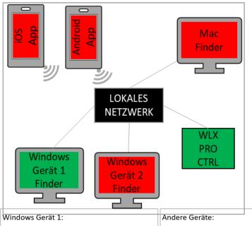
If the first device (Windows Device 1) is connected to the wAppLoxx Pro Control, a security key has been generated that is unknown to the rest of the devices. So that you can connect to the WLX Pro Control, the security key of the first device (Windows Device 1) must be shared. The initial key issue can be undone by pressing Reset D.
