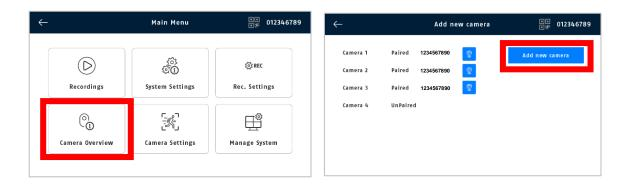
The camera supplied in the set is already programmed into the monitor at the factory. If you would like to pair a second camera, proceed as follows:
