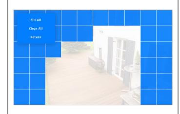
Here you can define the desired areas in which motion detection is desired. This helps you to minimise unwanted triggering. The areas marked in blue are the active areas. When triggered, a recording is started there.
