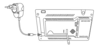
Unfold the stand and lock it in place by pushing it upwards. Then connect the supplied 12 V DC / 1 A power supply unit. Switch on the monitor using the on/off switch and follow the instructions on the monitor to complete the initial setup. Then connect the antenna to the monitor.
